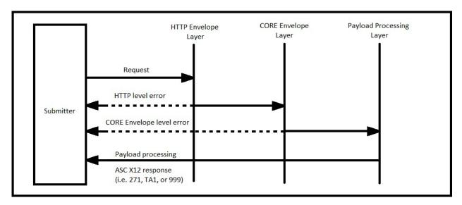
Note: The dashed lines represent error messages returned if an error occurs at the corresponding processing layer. The solid lines represent request/response messages.
