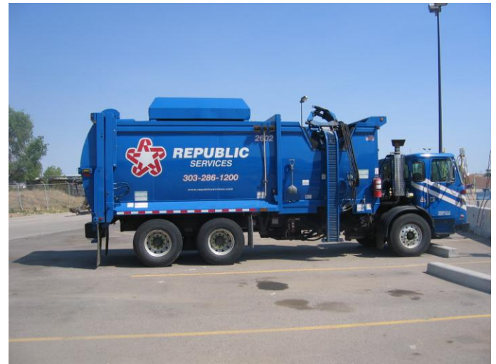
Truck configurations vary. Shown: automatic loading AutoCar chassis with McNeilus body
