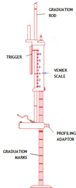
Figure 2. USGS Top Setting Wading Rod Components
