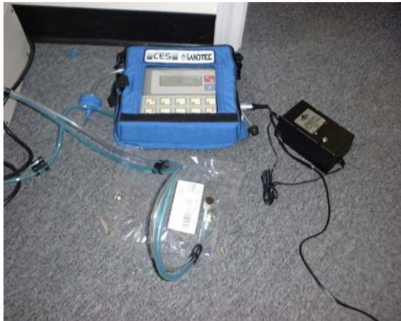
Figure 9. Analysis of O 2 , CO 2 , and CH 4
