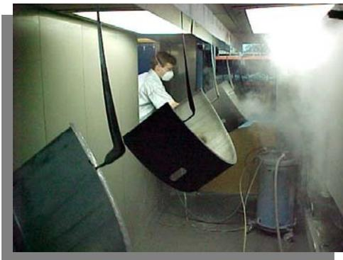
adhere to the surface of the grounded parts until they are melted and fused to the part by a curing process. Powder coating involves three steps: (1) pretreatment, (2) powder application, and (3) curing. Pretreatment is required to ensure an acceptable coating finish. Surface preparation usually involves alkaline cleaners, iron or zinc conversion coatings, and rinsing. Step 2, powder application, uses four types of equipment:
