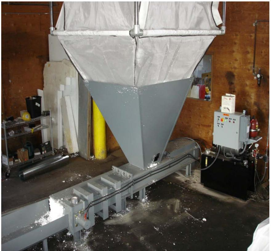
**Figure 1 – Densifier installation showing hopper, densifier cylinder, and catch tray for finished densified material.**
