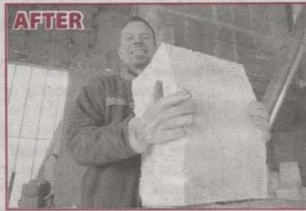
Thanks to a grant from the State of Colorado, Eco-Cycle has a new densifier that compresses bulky #6 white block foam to less than one-tenth its original volume, significantly reducing the financial costs and carbon footprint of transporting the material.
