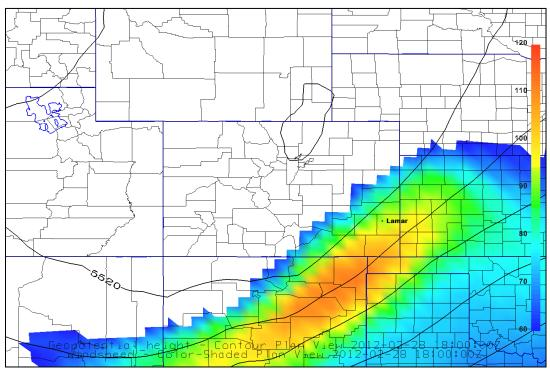
Figure 11: NARR 500 mb analysis for 18Z February 28, 2012, or 11 AM MST February 28, 2012 showing wind speeds in knots. Only speeds above 60 knots are shown. (Source: <a href="http://nomads.ncdc.noaa.gov/data.php?name=access#hires\_weather\_datasets">http://nomads.ncdc.noaa.gov/data.php?name=access#hires\_weather\_datasets</a>)
