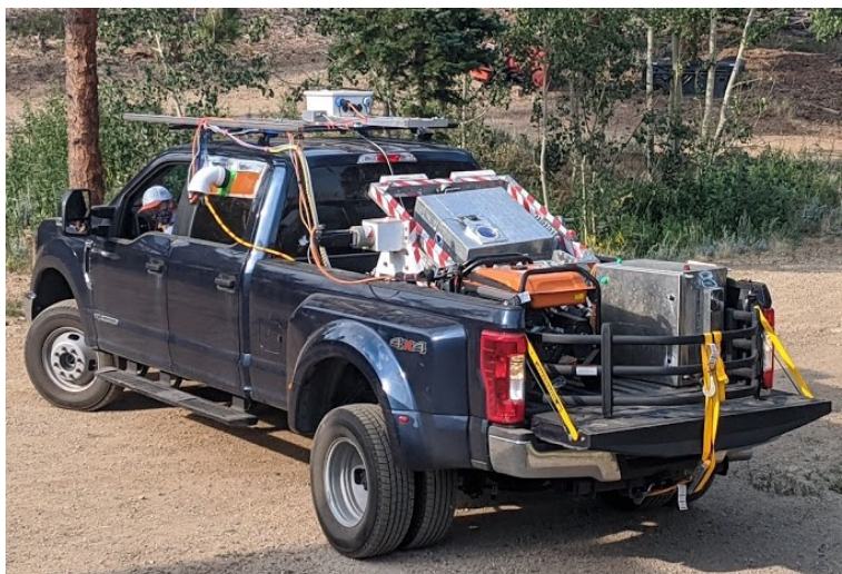
Figure 2: Photograph of NOAA’s Mobile Lidar Van, which provided spatial, temporal, and vertically resolved wind speed and wind direction measurements along the aircraft inflow and outflow flight legs.
